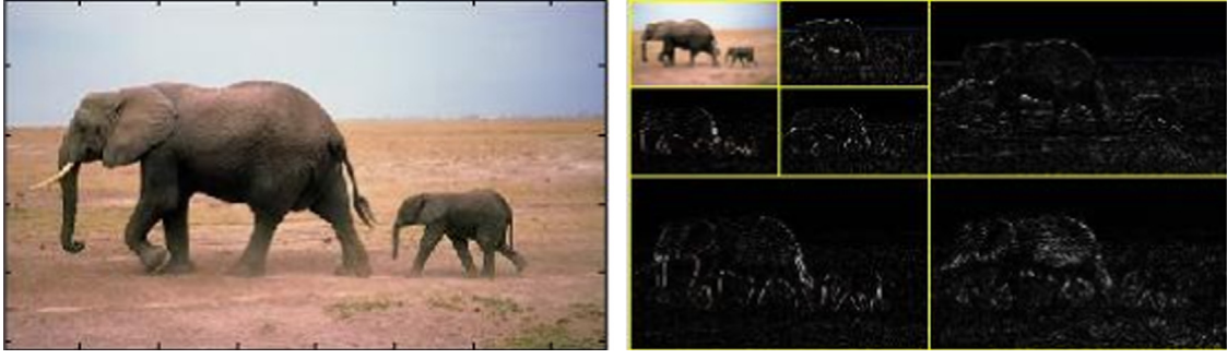
Fig. 3. Layout of individual bands at second level of DWT decomposition.
